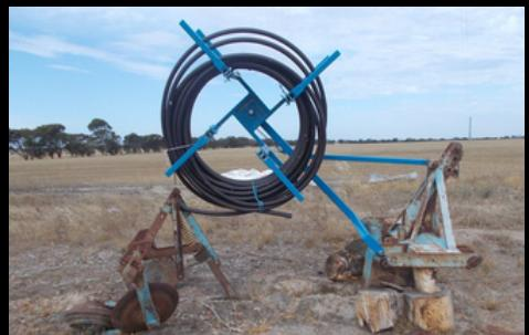
**RIPPER & PIPE LAYER with disc mounter for tree planting, press wheel + polypipe layer, handles 2-inch polypipe, plus spinning wheel.**
